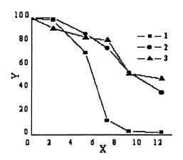
Figure. 1. The dynamics of change of the tracer contents in water. X - days of measuring; Y - content of tracer, %;  $I - \text{adding of } 50 \text{ mkM/l CdCl}_2$ ;  $2 - \text{acute } \gamma - \text{irradiation in a doze } 15 \text{ Gy}$ ; 3 - control
